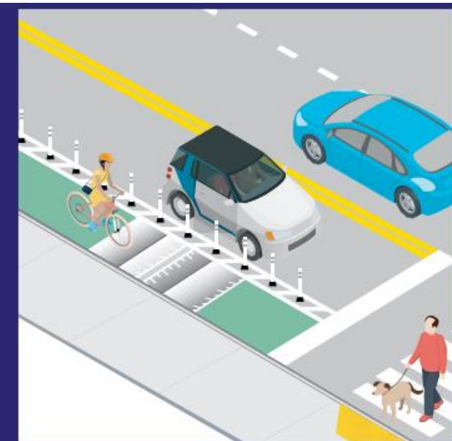
Figure 13. Speed bumps with drainage strips.
