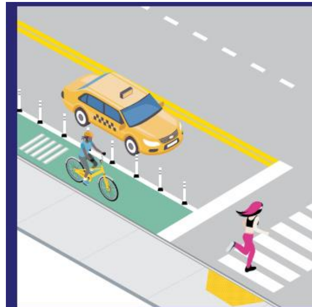
Figure 12. Rumble strips slow down bicyclists and alert riders to an upcoming pedestrian crossing.
