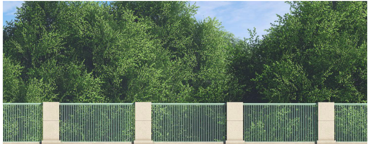
Concrete Post with Metal Handrail - Elevation
