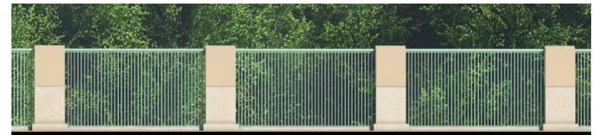
Concrete Post with Metal Handrail - Elevation
