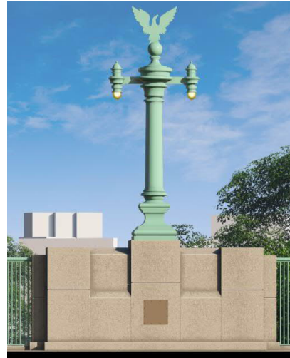
Elevation at Single Light Pole
