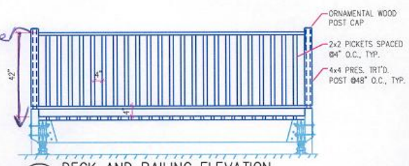
3 DECK AND RAILING ELEVATION SCALE: 1/2" = 1'-0"
